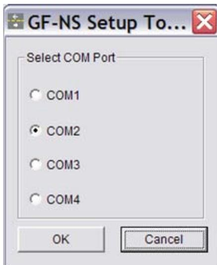
1. Select the COM Port of your computer that will be used to export the data to the GF-NS/A module. (COM2 is the default setting.)
