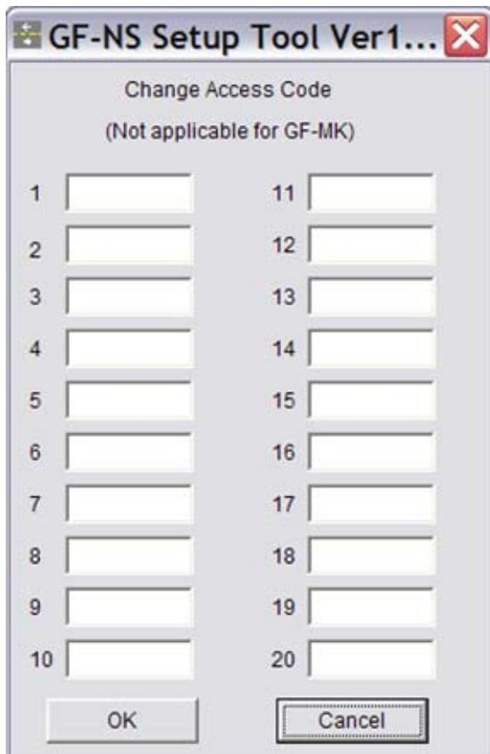
In each box, enter a 4-digit number. The program will not allow any other code length. Once saved and imported into GF-NS/A, any 4-digit number programmed here will activate the door release contact. The contact length can be set on the GF-DA/B module to momentary, or from 0.5 to 20 seconds.
