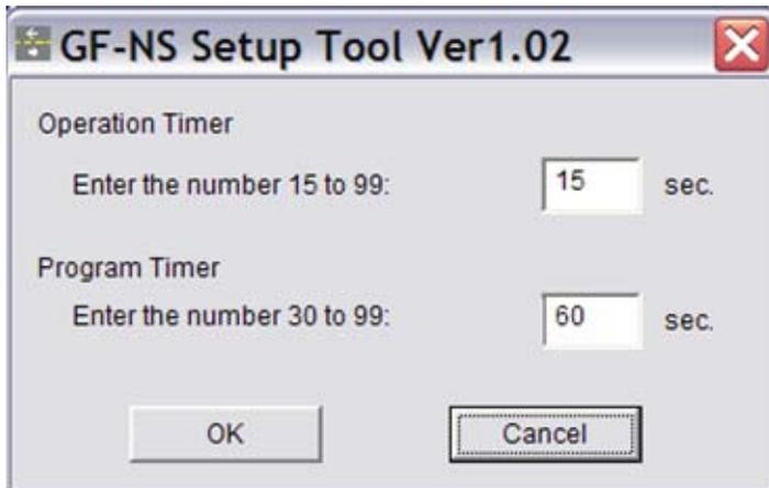
The screenshot shows a dialog box titled "GF-NS Setup Tool Ver1.02". It has two sections: "Operation Timer" and "Program Timer". Under "Operation Timer", there is a text input field containing "15" followed by "sec.". Under "Program Timer", there is a text input field containing "60" followed by "sec.". At the bottom, there are two buttons: "OK" and "Cancel".
