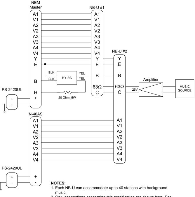
2. Only connections concerning this modification are shown here. For complete system installation, please refer to the NEM system instructions, included with the equipment.
