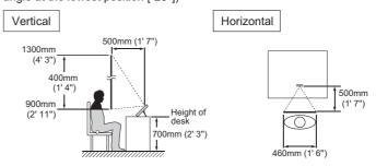
When installed on a flat desktop (with desktop stand at  $30^\circ$  and camera angle at the lowest position [-20°])
