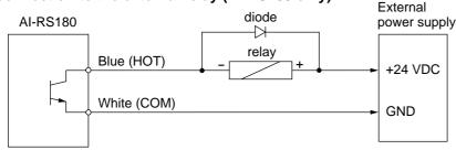
Note: AI-RS180 open collector output is 30 mA / 24 VDC (max.).
