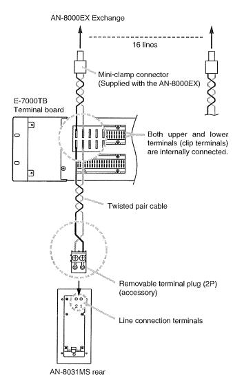
To connect the cables from the AN-8000EX Exchange to the AN-8031MS, use the removable terminal plug (2P) supplied with the AN-8031MS.
