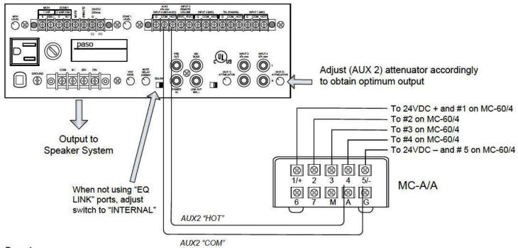
T3115BGM or T3130BGM with the PD-1 or PD-2 and TD-H System:
