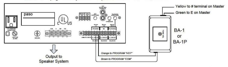
DMA2060 or DMA2120 with the BA-1 or BA-1P:
