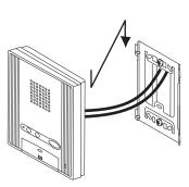
**3** Mount the station unit to the mounting bracket.
