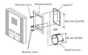
**1** Mount the mounting bracket on the 1-gang box or round back box.
