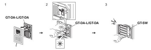
Press the call button assigned as the light button to light up the light connected to the entrance.
