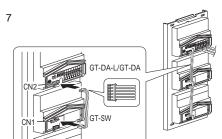
**7** From the speech module to the next module, insert the attached connector into the socket.
