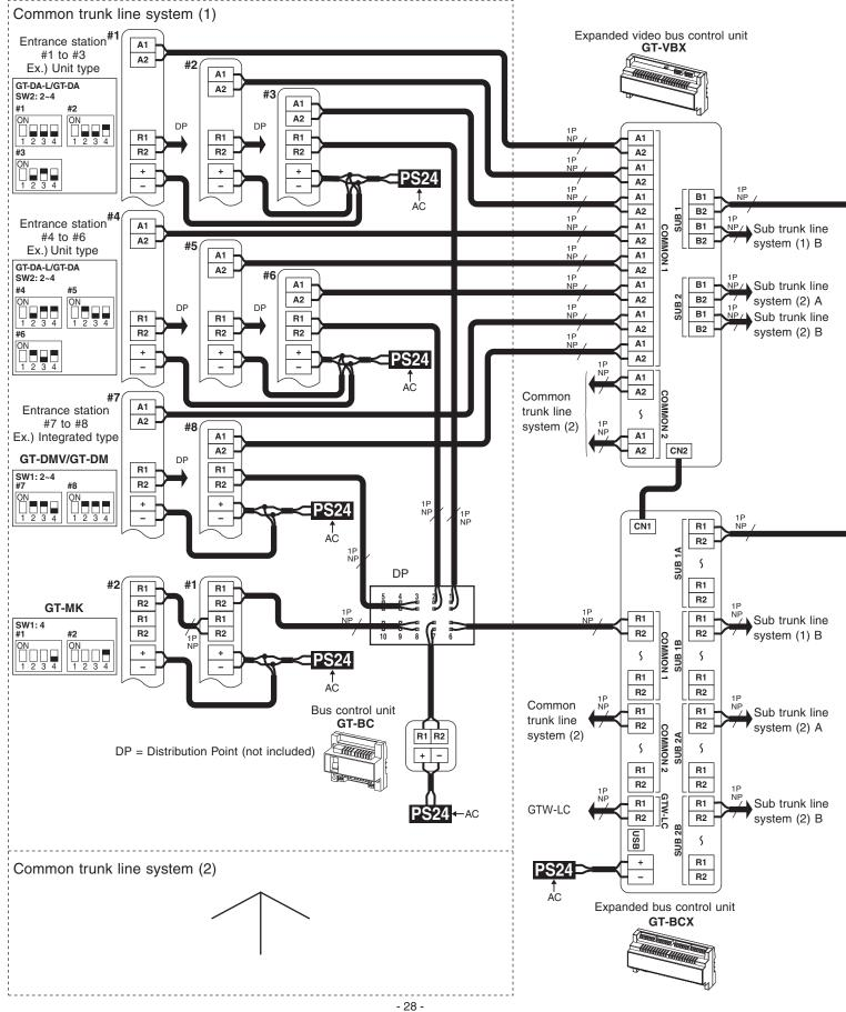
⚠ Put each piece of wiring in a separate sheath as shown in the diagram below.
