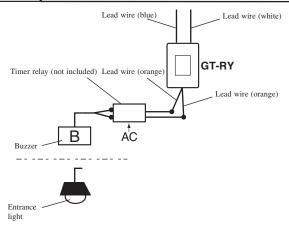
\* When the GT-RY is connected, the separate option connecter (4-5) is required.
