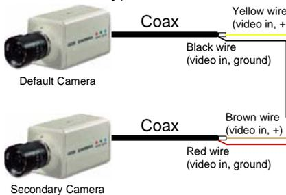
If only using 1 CCTV camera, connect it to the Yellow and Black wires. The secondary camera to the Brown and Red wires will be used if you desire another camera in the lobby area and the ability to switch between the two cameras.
