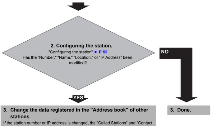
If the station number or IP address is changed, the "Called Stations" and "Contact Input Call" settings of the door station should also be changed. (IX-DA, IX-BA)
