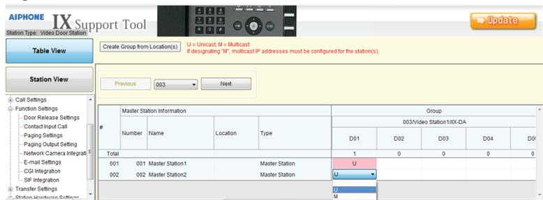
Select **Contact Input Call** again from the menu on the left. Using the drop down under Group Number, select the group that was created in the previous step. Using the drop down under Priority, select the priority level at which the mushroom button is to place a call (figure 5). Press the Update button to save changes.
