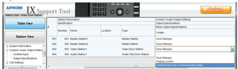
In order for the mushroom button push to be able to call the master(s), a door station group will need to be created. Expand **Function Settings** from the menu on the left and select **Contact Input Call**. Click on the **Open Door Station Group List** button at the top of the page (figure 3).
