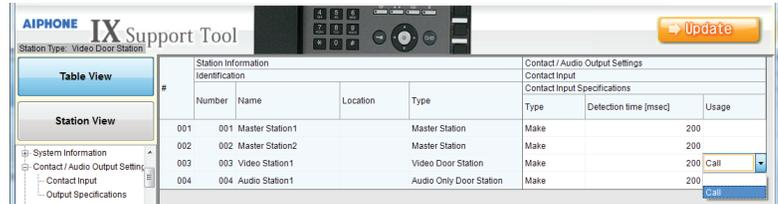
The contact output specifications will need to be set for contact input call / communication state. Select **Output Specifications** from the menu on the left. Use the drop down under "Usage" and select **Contact Input Call / Communication State** for the appropriate station (figure 2). Press the Update button to save changes.
