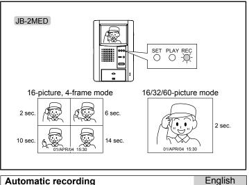
If a call is received from the entrance, the unit starts recording automatically. The REC button lights during recording.
