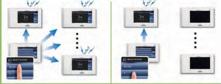
Easily communicate between stations. Simultaneously make an announcement to all inside stations or select a single station to call.
