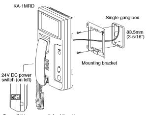
Turn off this power switch while wiring.
