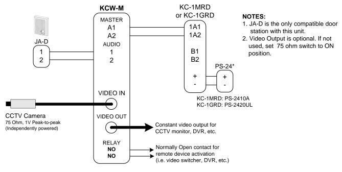
When VIDEO OUT is connected, set 75 Ohm switch to OFF position.
