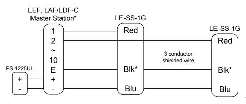
\* In a single master LEF system only, 2 conductors homerun can be used with the BLK and BLU wires tied together and "E" and "-" jumpered at the master station.
