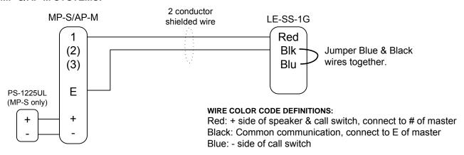
Intercom wiring must be run at least 20" away from any AC wiring, fluorescent lighting, dimmer switches, or any other electronic device that may cause interference.
