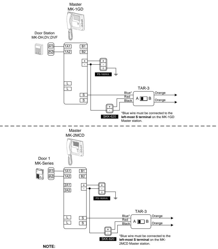
The TAR-3 provides a closure with each stroke of the chime from the monitor. (i.e. Four closures during a four-stroke chime sequence.) If a single momentary contact is required, please refer to modification #RELAY 1198-902.
