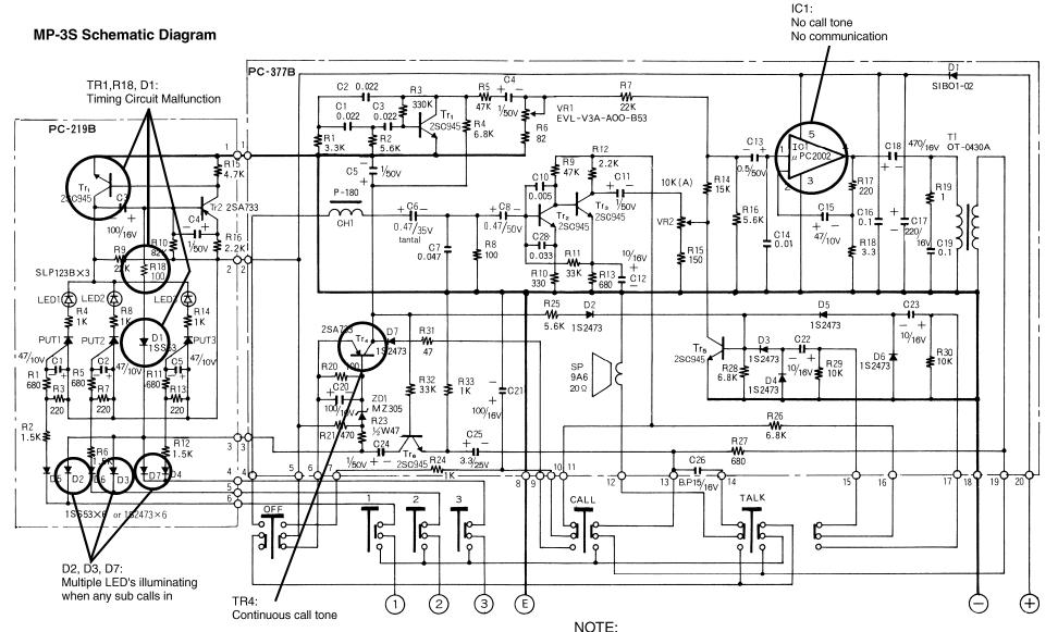
The components marked have the potential for being damaged by a power surge. Actual damage caused depends on the severity of the surge.
