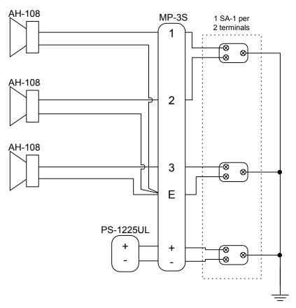
To Earth ground (Cold water pipe or equivalent. Do not use electrical ground.)
