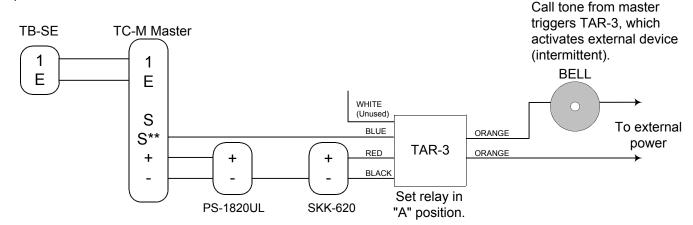
\*\* Connect the BLUE wire to the "S" terminal at the BOTTOM of the terminal strip. Verify correct terminal with an continuity meter, using the S terminal that is not connected internally to the "E" terminal.
