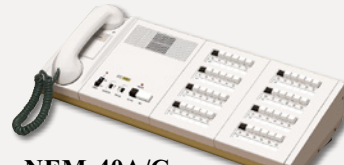
NEM-40A/C 40-Call Handset Audio Master Station 10-1/4" H 23-7/16" W 6-15/16" D
