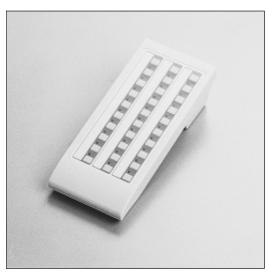
The NHX-30G 30-Station Add-on Selector expands the CommuniCare system to its maximum capacity of 80 stations. With a simple connection to the NHX-50M, the 80-call master station remains streamline and compact in size.
