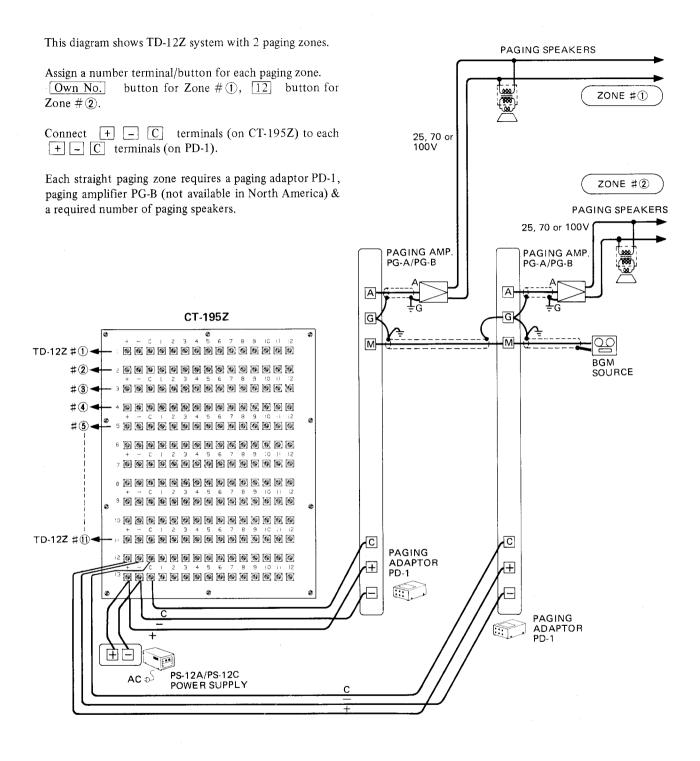
Installation of paging zone (with or without talkback) reduces one station capacity of TD-Z system.
