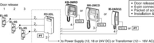
Run door release wires in separately jacketed cable from audio/video wires.
