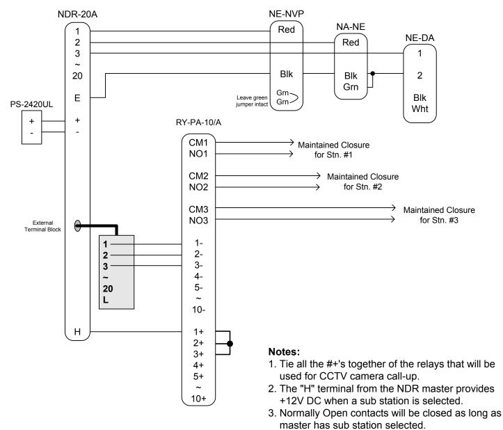
4. Only wiring concerning door release is shown here. For complete system information refer to the system installation manual.
