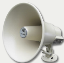
AH-16TN Horn Speaker • 8Ω, 25/70V, 16W • Indoor or outdoor use • Surface mount Bell Diameter: 8-1/4" Depth: 9"
