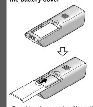
Do not trap the connector of the battery
